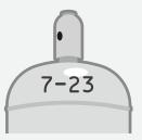
This figure shows that the cylinder passed the pressure test in July 2023. Since it has not been 5 years since the test, the cylinder has not passed its expiration date.
