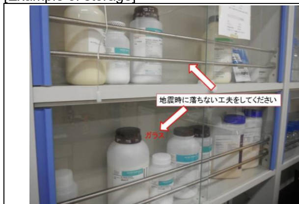
Use bars or glass panes to prevent containers from falling in the event of an earthquake.
