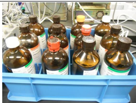
Prevent bottles from contacting each other in the event of an earthquake.
